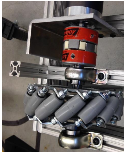
Figure 25. Mecanum wheels, bearings, and collars.
