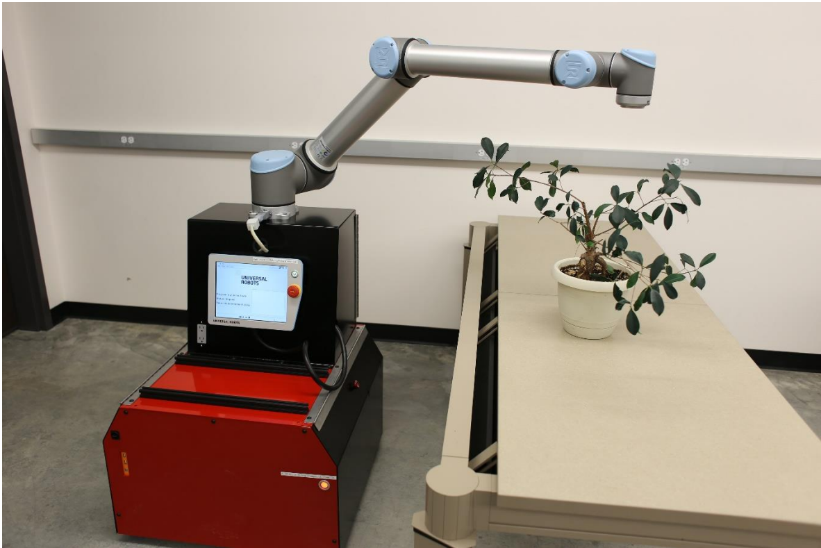
Figure 31. Finished rover, without end-effector sensors (optional).
